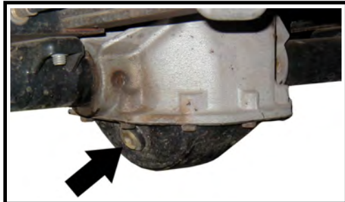
Level Plug viewed from in front of the right rear wheel
