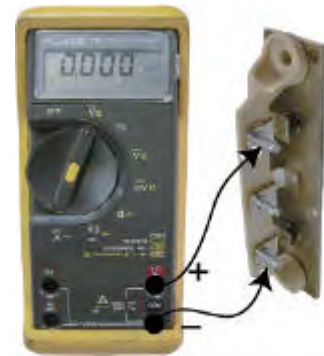
Transformer Secondary Circuit
