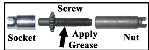
Brake Adjuster Assembly
