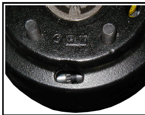
Brake drum shown with the access slot aligned with the adjusting star wheel .
