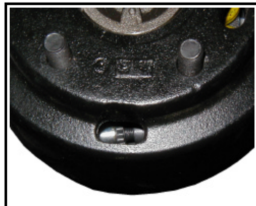
Brake drum with adjusting slot aligned with star wheel
