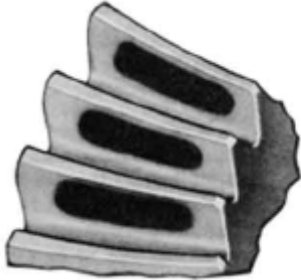
Ideal contact pattern Correct shim Correct backlash
