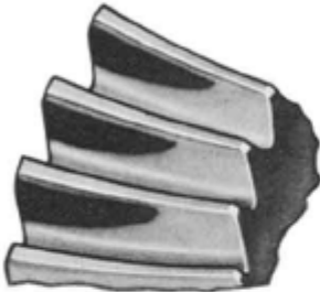
Backlash is correct Subtract 0.004" shim
