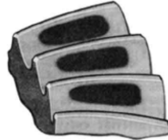
Ideal contact pattern Correct shim Correct backlash
