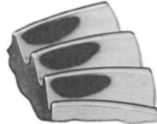
Backlash is correct Subtract 0.004" shim
