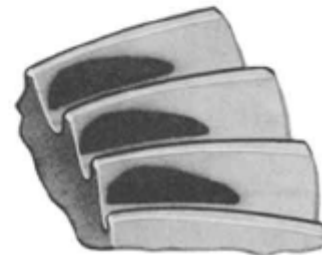
Shim is correct Increase backlash 0.004"
