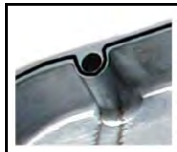
Apply sealer around the ID of the holes
