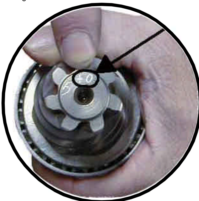
Number on face of pinion gear
