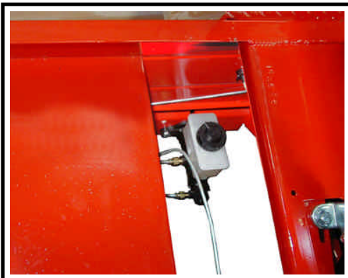
Master cylinder is located between the front seats. Dual reservoir shown.
