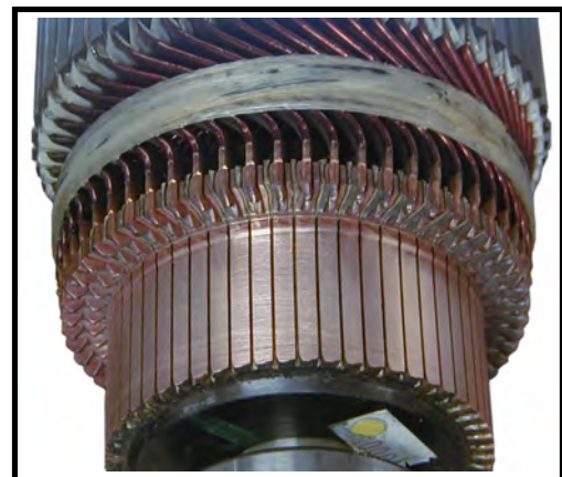
Example of freshly cut commutator
