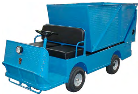
B 2-48-36 Equipped with optional hydraulic dump bed
