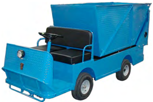
B 2-48-36 Equipped with optional hydraulic dump bed
