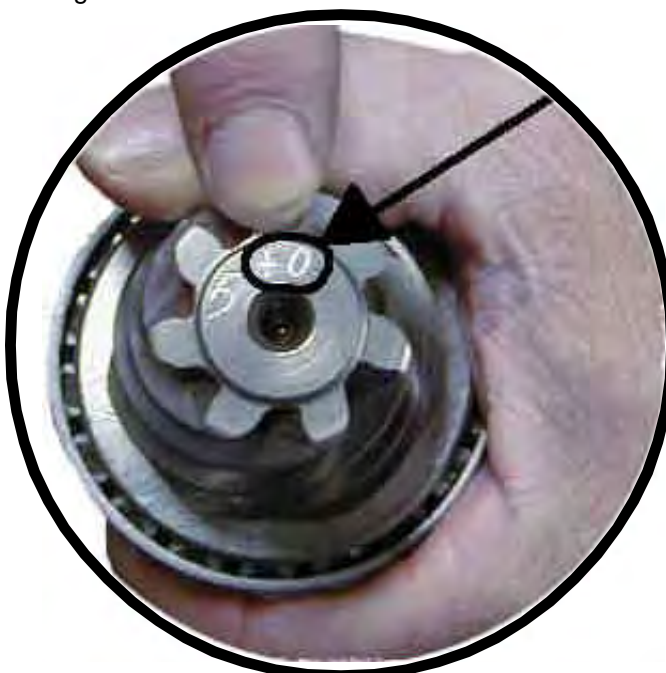
Number on face of pinion gear
