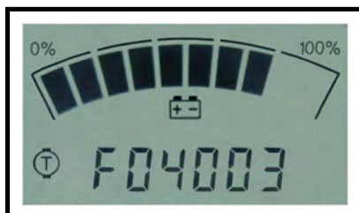
Display showing a fault code
