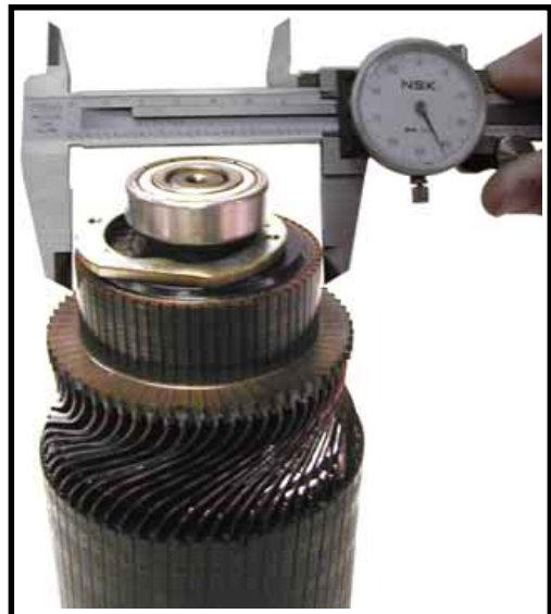
Example of freshly cut commutator
