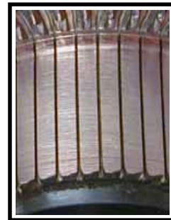
Properly undercut and cleaned commutator segments
