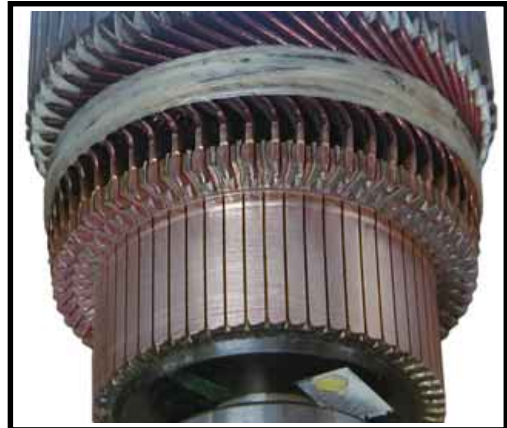
Example of freshly cut commutator
