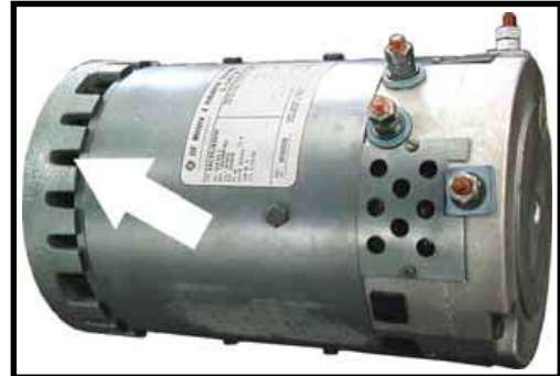
Typical motor with cooling fan indicated by the arrow
