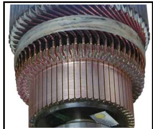
Example of freshly cut commutator
