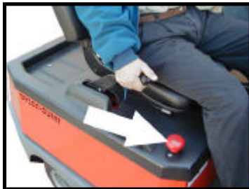
Emergency Battery Disconnect/Stop Switch
