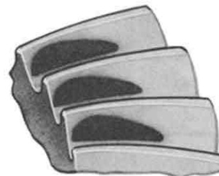
Shim is correct Increase backlash 0.004"
