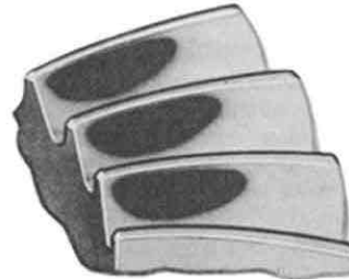
Backlash is correct Subtract 0.004" shim
