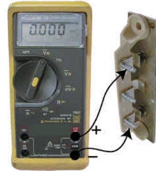
Transformer Secondary Circuit
