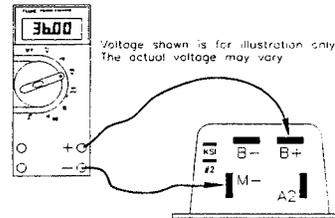
Measuring Voltage Across B+ and M- of PMC: The correct meter reading should equal the battery voltage at time of test.
