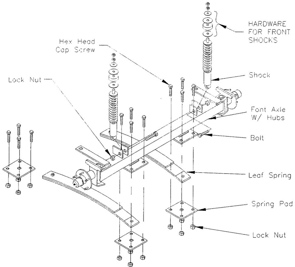
**Front Axle Figure 1: Front Axle and Suspension**
