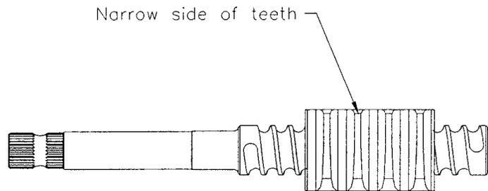
**Front Axle Figure14: Worm Shaft**
