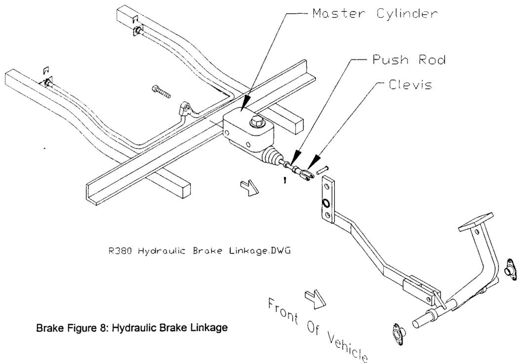
Brake Figure 8: Hydraulic Brake Linkage
