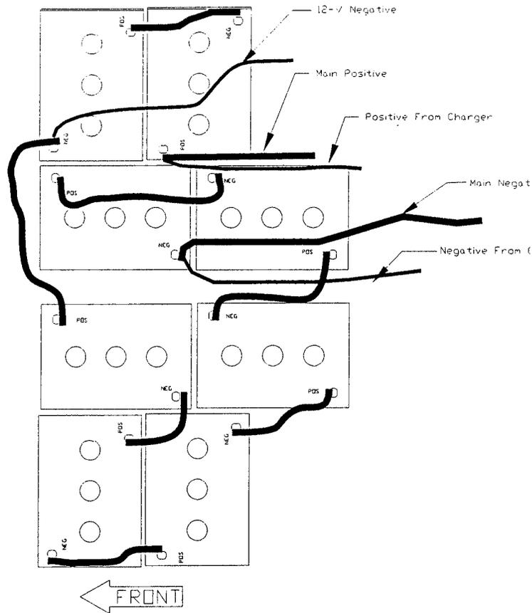
**Battery Configuration:** Shown are the batteries and how they are connected together for 48-Volt electrical system. The battery configuration for the 36-Volt system is shown on page 3-63.
