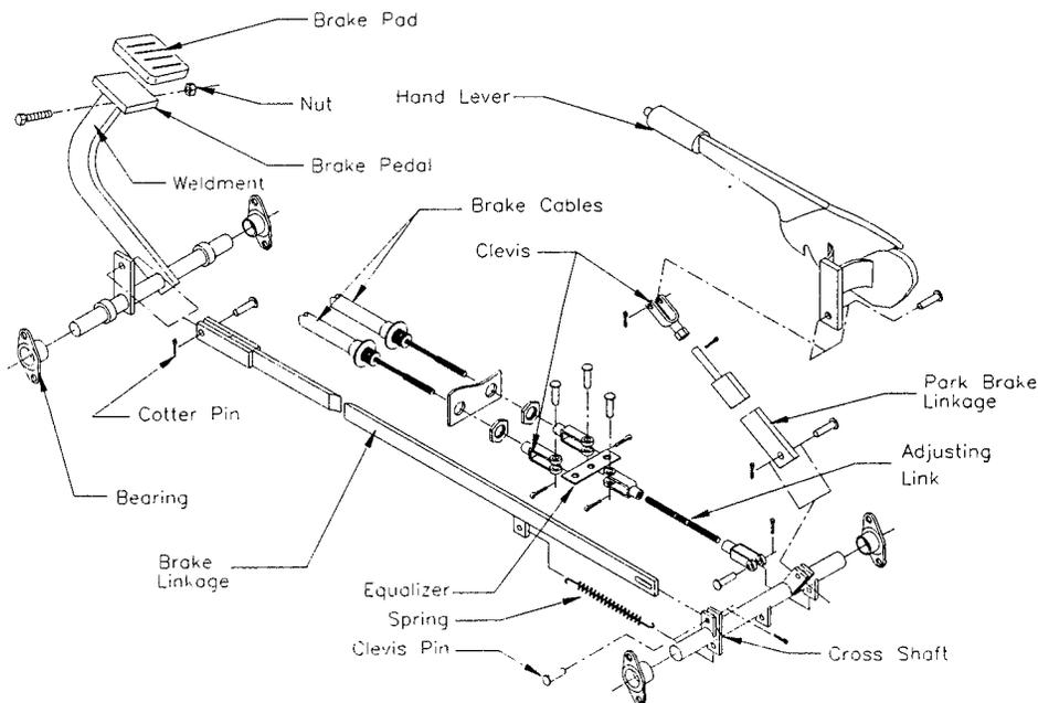
Brake Figure 3: Brake Linkage
