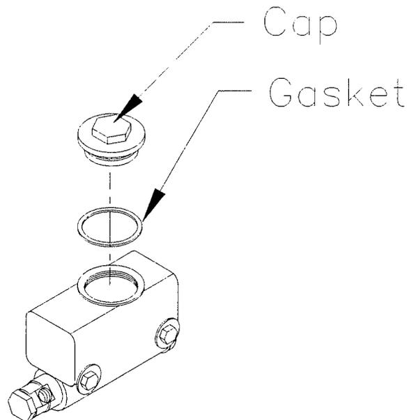
Brake Figure 7: Filling Master Cylinder
