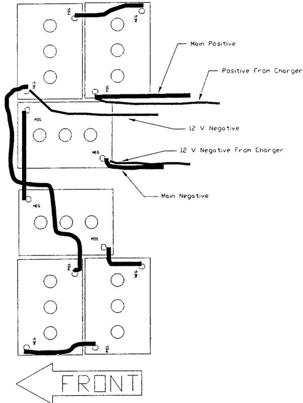
**Battery Configuration:** Shown are the batteries and how they are connected together for 36-Volt electrical system. The battery configuration for the 48-Volt system is shown on page 3-64.
