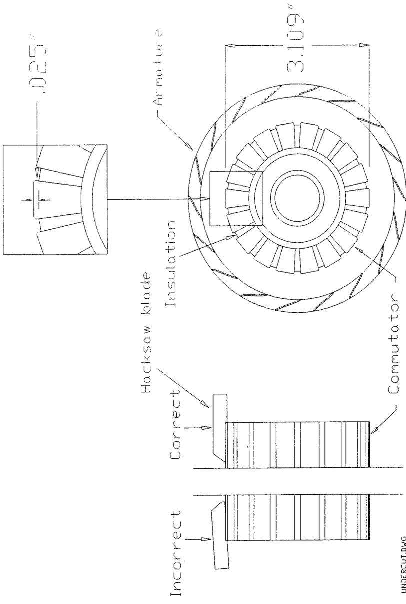
Undercut Figure: The left side shows how to properly cut the mica using a hacksaw blade. The right side of the figure shows
