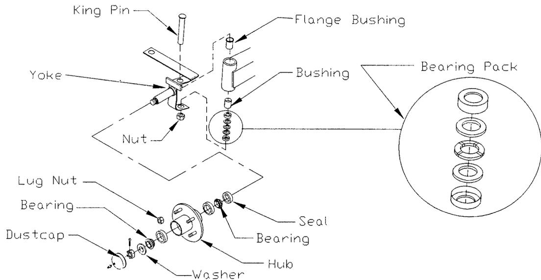
**Front Axle Figure 4: Yoke Assembly**
