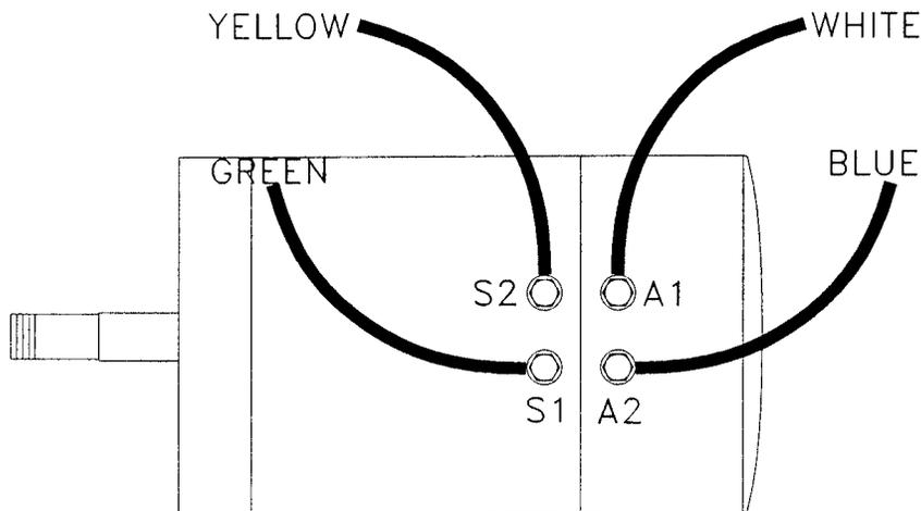
**Typical wire connections on motor:** In this figure we show the wire connections to the motor and their colors. Be sure to label each of the wires with their correct locations before removing them from the motor.
