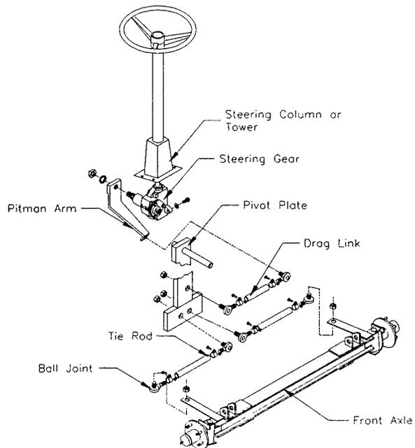
**Front Axle Figure 12: Complete Steering Assembly**
