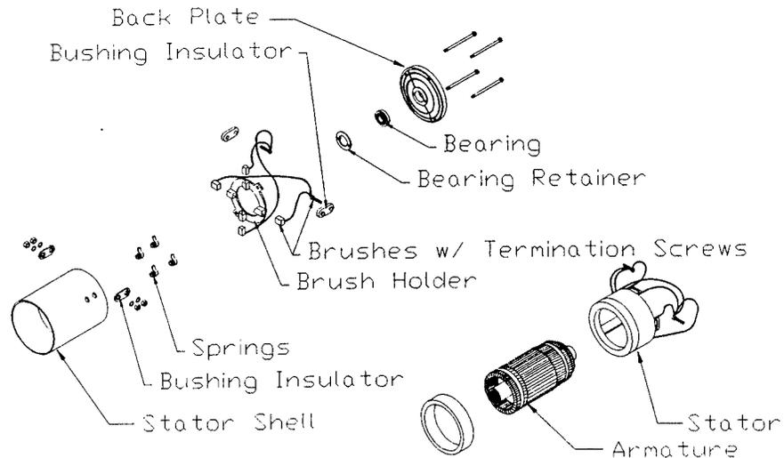
**Exploded View of the 70-049-05 Motor.**
