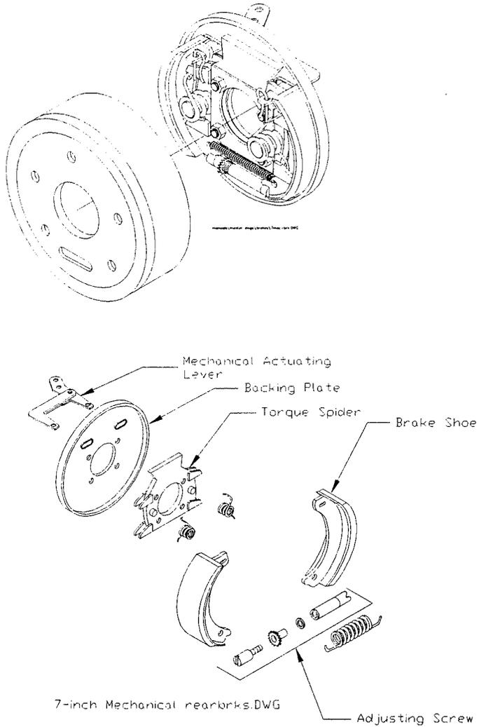
Brake Figure 1: Mechanical Brake
