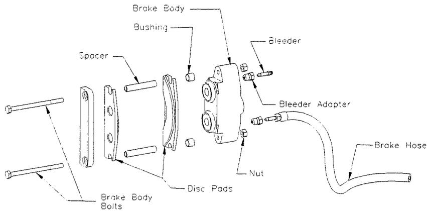
Front Hydraulic Disc Brake Body.
