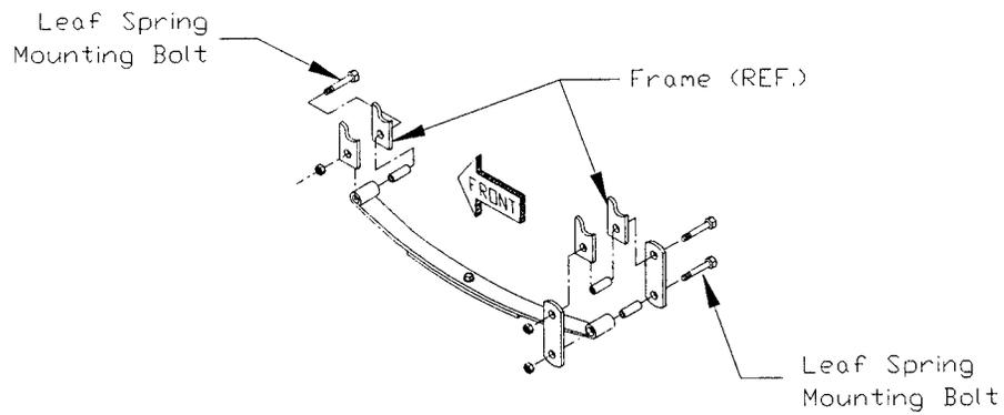
**Drive Assembly: The drive assembly is mounted to the frame by the leaf spring**
