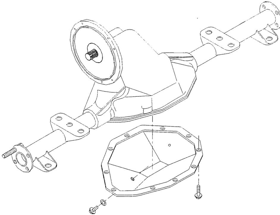
**Differential:** The differential case cover is removed to drain the oil. When replacing the cover the bolts must be torqued to 16-24 ft-lb.
