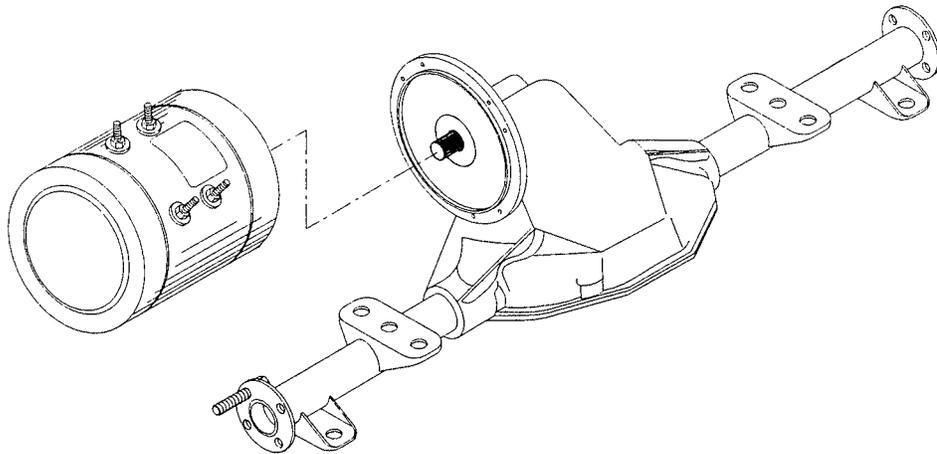
**Motor removed from the drive assembly:** The motor is easily removed by disconnecting the wires and removing the mounting bolts. Be sure to support the motor before removing the bolts.
