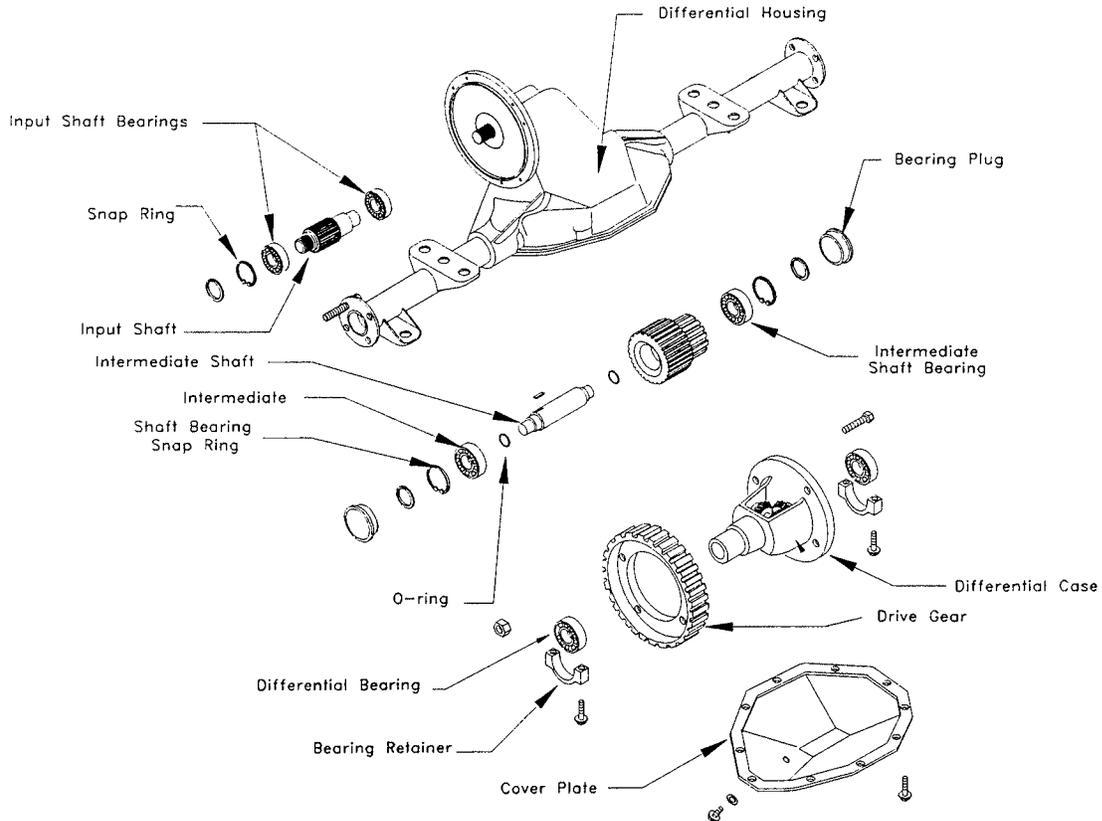
**Exploded view of the differential assembly: This view shows the parts contained with in the differential. Part numbers are available in the Illustrated Parts section of this manual.**
