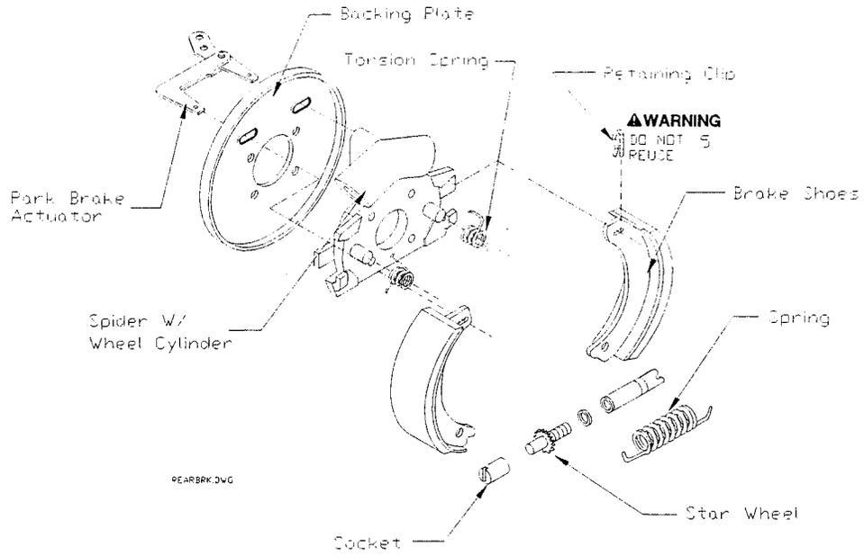
The Star Wheel and The Adjusting Slot on the brake drum must be lined up in order to make adjustments
