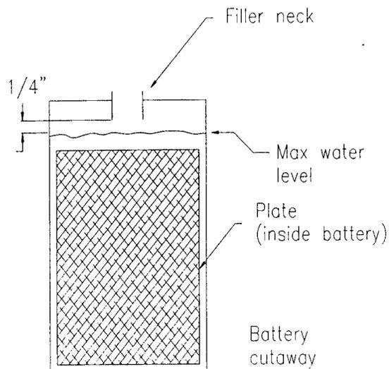
**Battery Fill Level: This figure show the proper fill**
