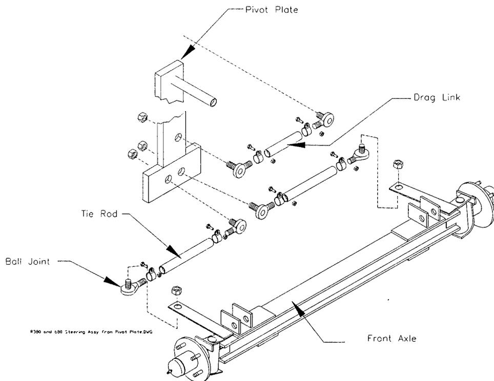
**Front Axle Figure 8: Steering Components**
