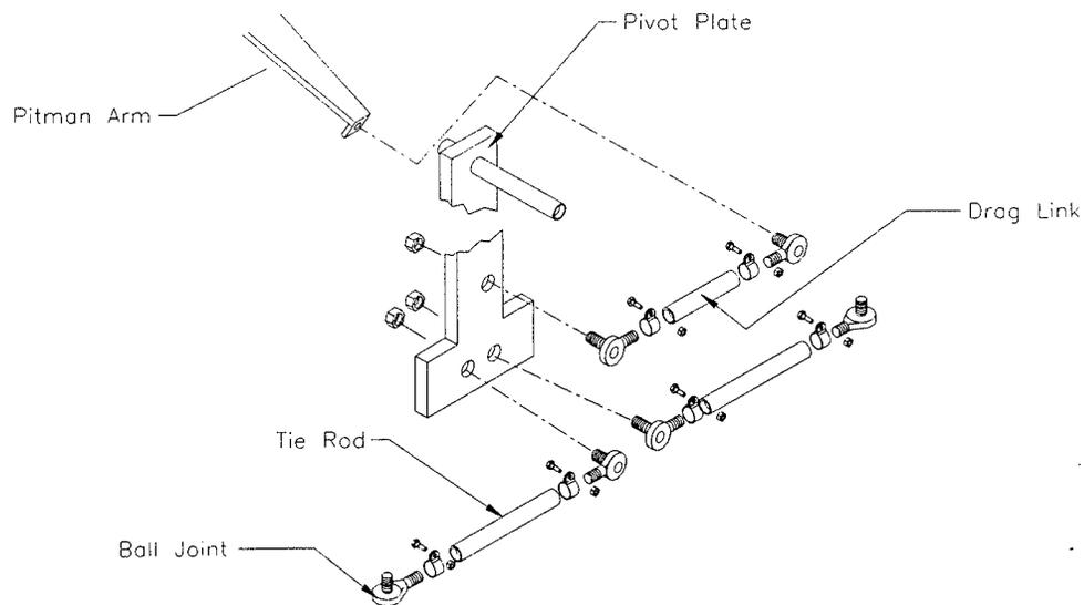
**Front Axle Figure16: Ball Joint and Drag Link**
