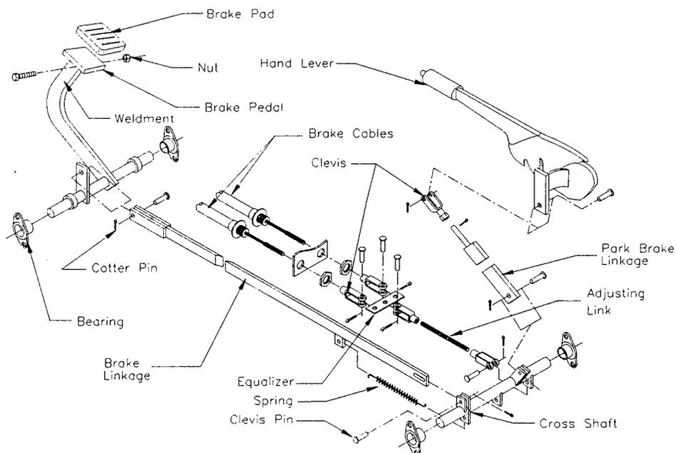
Brake Figure 2: Mechanical Brake Linkage
