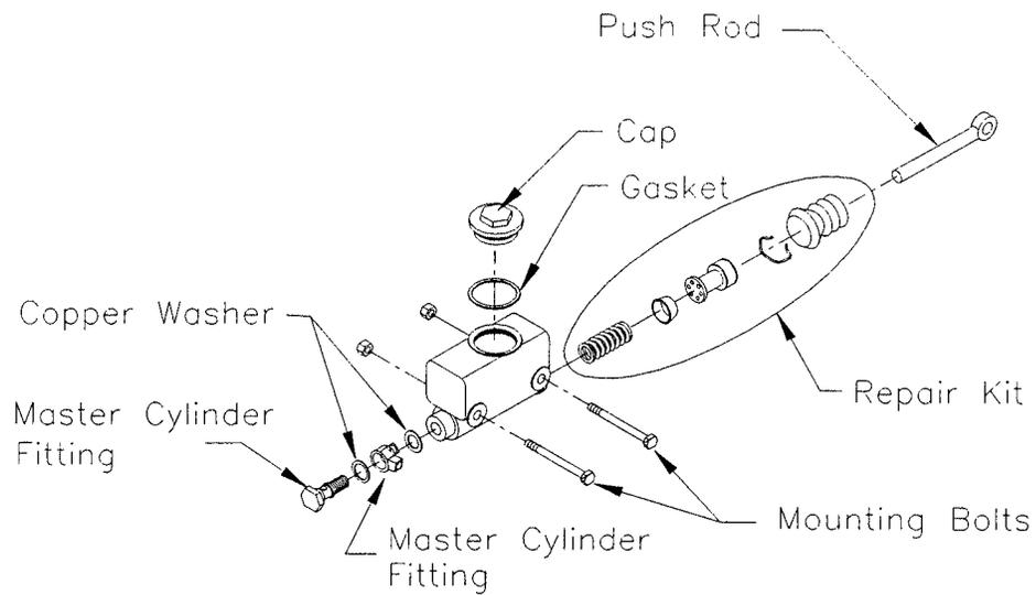
Brake Figure 6: Master Cylinder
