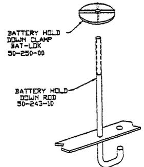
INSTALLATION OF BATTERY HOLD
