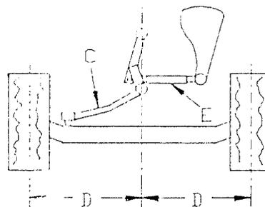
4. Return vehicle to ground for turning load. Center steering mechanism by turning steering wheel full clockwise. Counting number of full turns, turn steering wheel full counter clockwise. Counting half the number of full turns return steering wheel to center. Install 18-040-11 (E) adjust so steering wheel is stopped by internal gear box stops in both directions of wheel turn.
