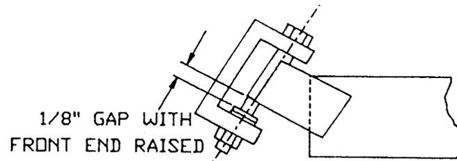
2. Adjust connecting arm on front axle for proper toe-in of 0 to 1/8 inches.
