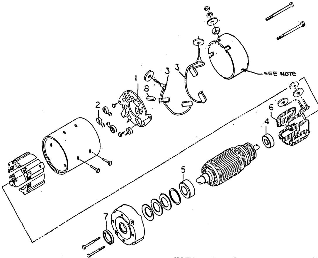
NOTE: Brush measurement holes (2). With new brushes a 1/16" drill rod can be inserted approximately .780" into the brush measurement holes. Brushes should be replaced when rod can be inserted 1.560" into hole. This leaves approximately 1/8" wear remaining.
