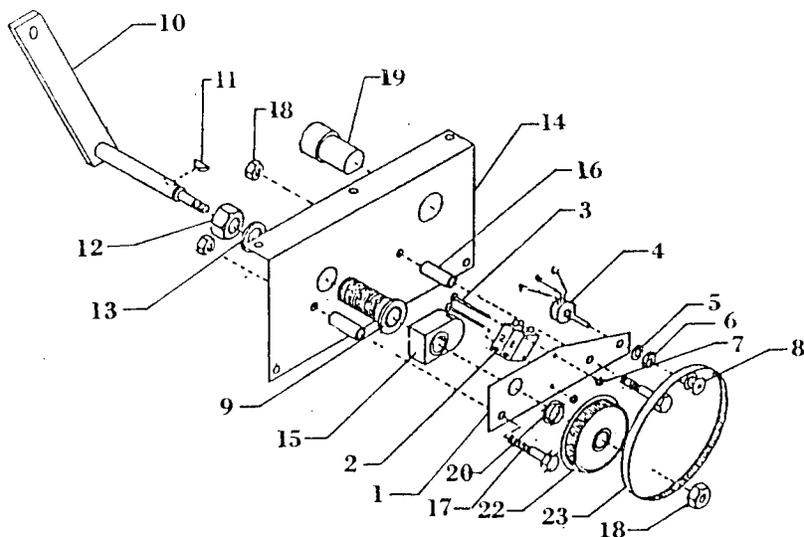
ACCELERATOR MODULE (COVER NOT SHOWN) 62-030-14, MODEL R 3-80
