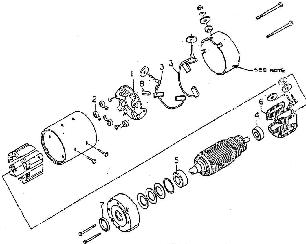
NOTE: Brush measurement holes (2). With new brushes a 1/16" drill rod can be inserted approximately .780" into the brush measurement holes. Brushes should be replaced when rod can be inserted 1.560" into hole. This leaves approximately 1/8" wear remaining.
