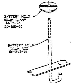
INSTALLATION OF BATTERY HOLD
