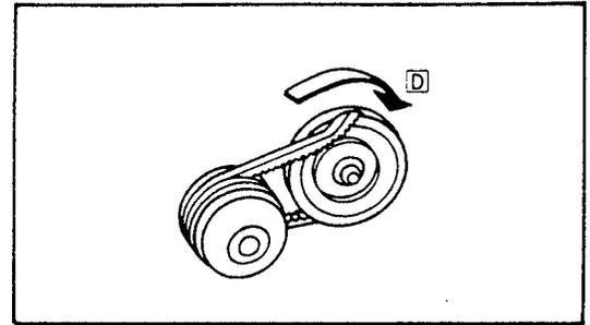
6. Rotate the secondary sheave clockwise: D and the belt will roll off the secondary sheave.
