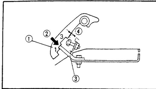
3. Measure the position of acceleration pedal just as the carburetor begins to open, 4; using a ruler, 5, as shown.
