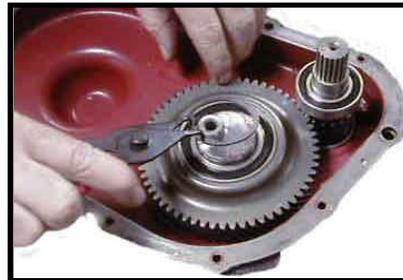
13. Remove the input shaft/bearing assembly and idler gear/bearing assembly from the gear case cover at the same time.
