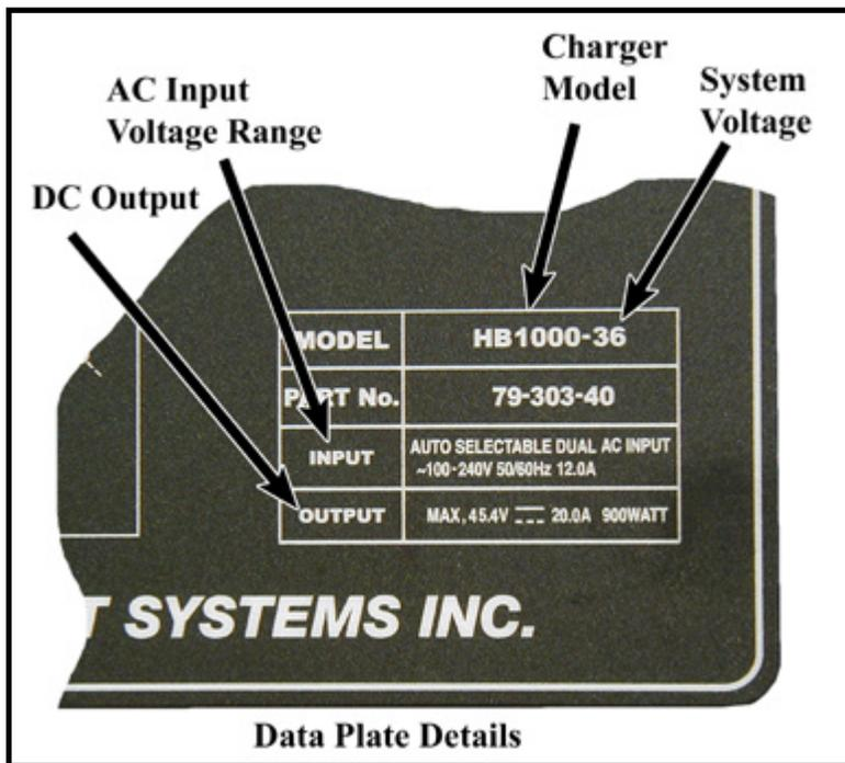
The model HB600W<sup>®</sup> and HB1000W<sup>®</sup> chargers are designed as semiautomatic chargers. The charger turns itself on when it is plugged into the wall outlet and turns off when the batteries are fully charged.
