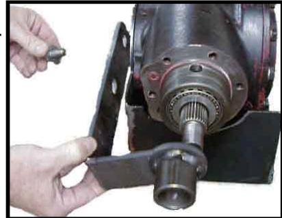
15. Check the gear lash between the ring and pinion gears. The gear lash should be .005 to .007 inches.
