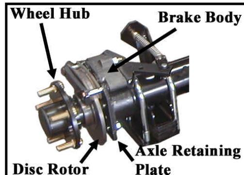
11. Remove the axle retaining plate and brake body assembly as one unit.
