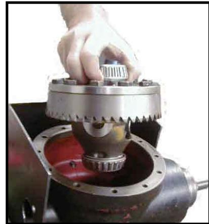
9. Pre set the carrier bearing preload by tightening the housing carrier bearing race ring nut until it requires 1.5 to 3.3 ft-lbs to rotate the differential assembly.
