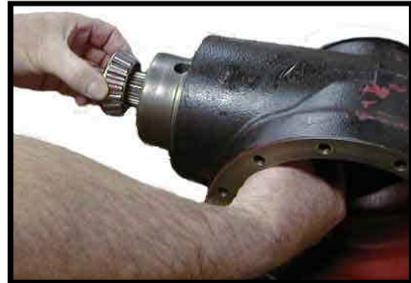
19. Remove the input shaft's shims and spacer.
