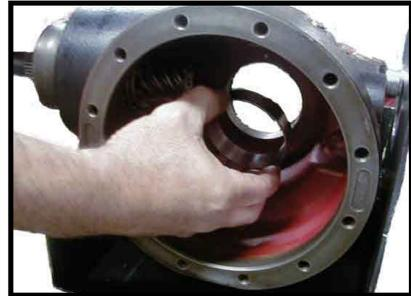
18. Remove the front bearing from the input shaft.
