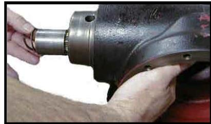
20. Remove the pinion shaft from the 3rd member.
