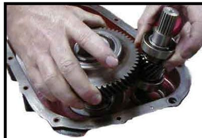
14. Remove the pinion nut from the output gear and remove the output gear from the pinion shaft.
