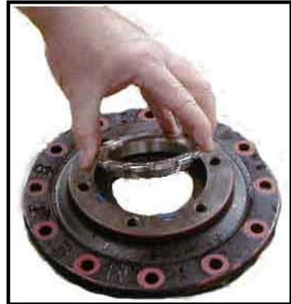
14. Turn the side plate over and remove the carrier bearing race from the side plate.
