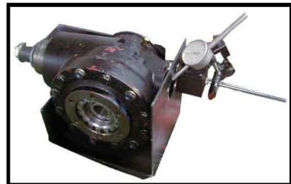
*NOTE: To move the ring gear closer to the pinion: Loosen the housing carrier bearing race ring nuts and tighten the cover carrier bearing race ring nut equally.*
