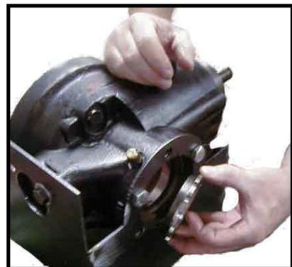
17. Remove the carrier bearing race from the 3rd member housing.
