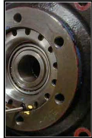
12. Install the pinion gear holding tool (96-500-42) and tighten the pinion nut enough to keep the pinion gear from rotating.
