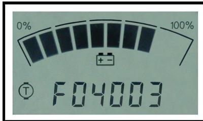
**Speed controller status:** The display will indicate a fault code whenever the control system logic detects a problem with the control system. A fault code is being displayed whenever the Fault Code Indicator (the letter ‘F’) is visible at the left of the numeric display. Refer to the table below for a list of fault codes and their descriptions.
