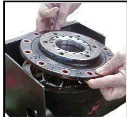
10. Mark the position of each carrier bearing ring nut in relation to the drive housing and cover and then remove the differential assembly, do not allow the ring nuts to rotate.
