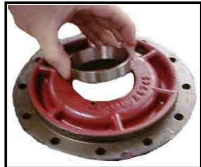
15. Remove the differential assembly from the 3rd member housing.
