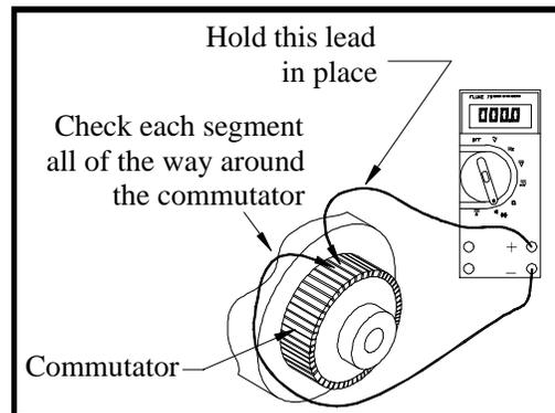
10. Using the continuity function of digital multi meter, check the continuity from any one of the commutator segments and the armature frame. If it is not an open circuit, then the armature is shorted and the motor must be replaced.
