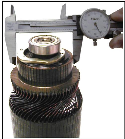
5. Thoroughly clean all copper debris from between the commutator segments.
