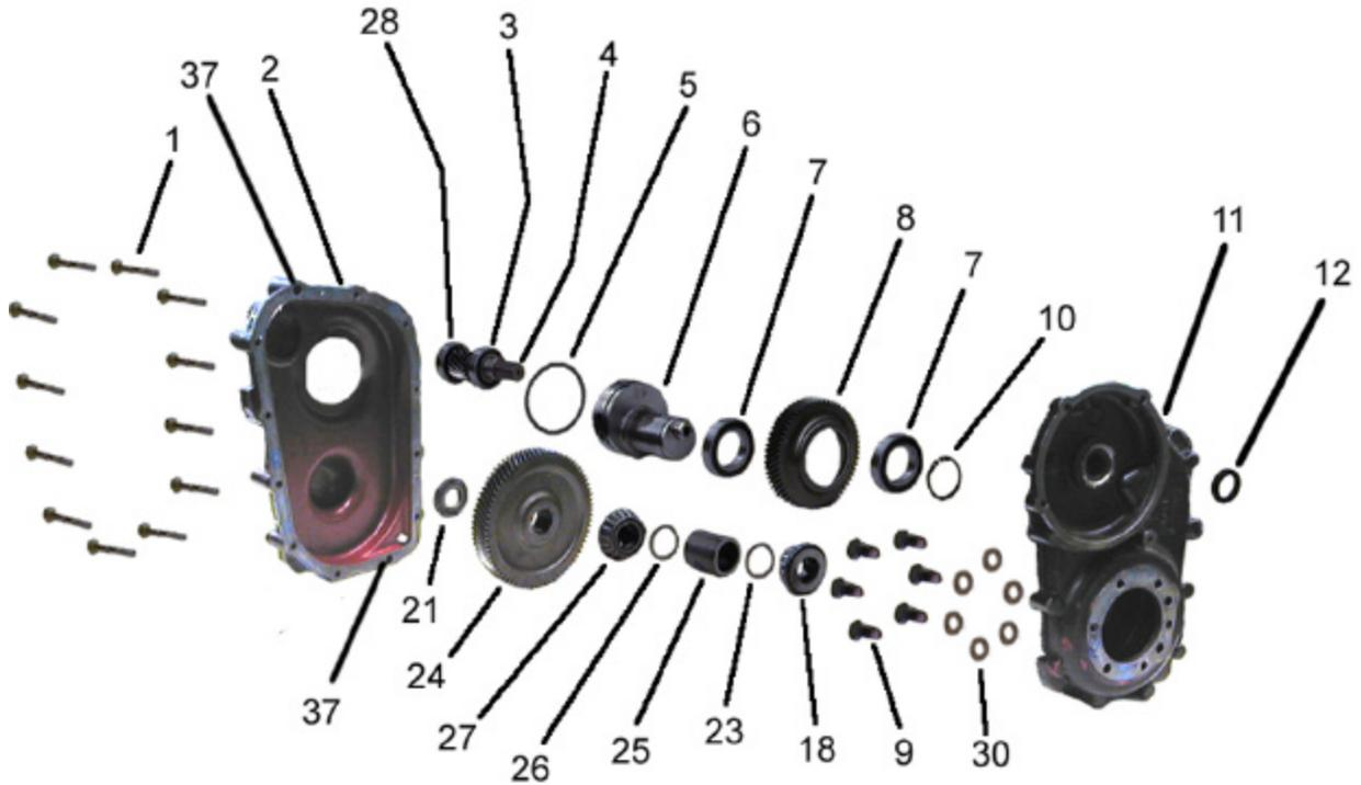
*Note 1: Spacer 23 is available in increments of .05mm starting at 3.9mm. 3.9mm spacer is part number GT-3287213. Add 10 to the part number for every 0.05mm over 3.9. For example, if 4.55mm is needed:  $4.55 - 3.9 = .65\text{mm over}$ ,  $0.65 / .05 = 13$ ,  $13 * 10 = 130$ . Part number for 4.5mm spacer is  $3287213 + 130 = 3287343$ .*
