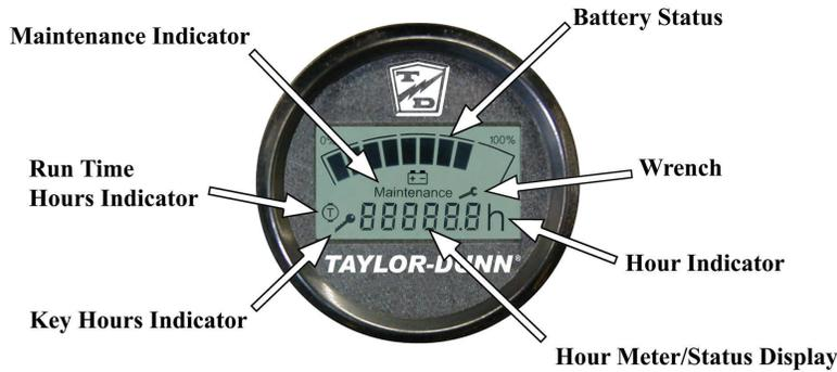
The Smart View Display (SVD) functions as a Battery Status Indicator (BSI), Hour Meter (HM), speed controller status monitor, and as an optional maintenance monitor feature. The operation of each of these functions is listed below.
