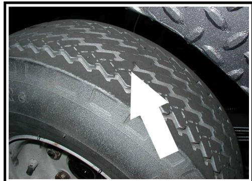
8. Inspect for uneven tire wear on the front tires. Uneven tire wear could be a result of an improperly inflated tire or a misaligned or damaged front end.
