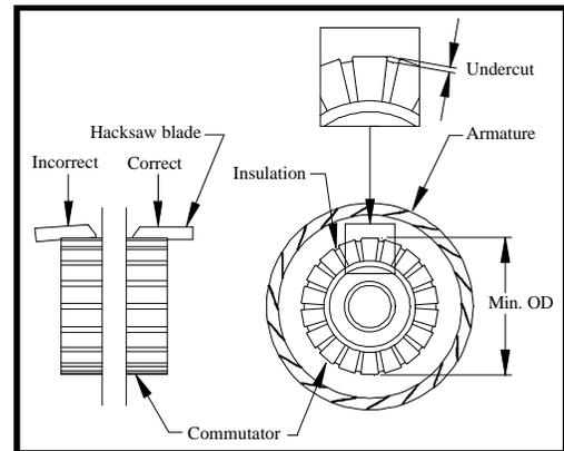
3. Inspect the armature for shorts. Refer to **Motor Inspection** section for information on testing the armature.
