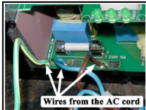
If both the AC and DC tests are good then the charger has failed. There are no internally serviceable components in the charger. If the charger has failed then it must be replaced.
