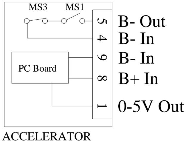
*Internal wiring shown for reference only. There are no internal serviceable components.*
