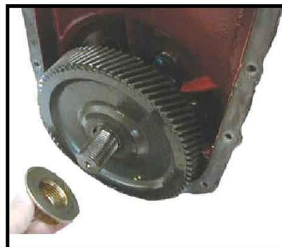
15. Mark the gear case position in relation to the 3rd member housing so that it will be reassembled in the same position.
