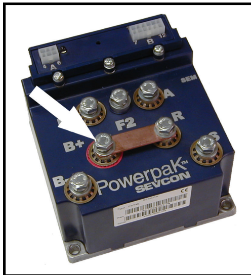
B+ Terminal on the Sevcon controller
