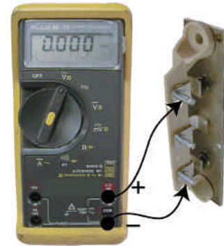
Transformer Secondary Circuit
