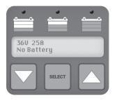
If the battery test is still unsuccessful, the charger continues to check the voltage on the battery cables until it detects an acceptable condition. If the test is successful, the battery charger displays the battery voltage before starting the charge, then displays the current value ( $\mathbf{A}$ ), the voltage ( $\mathbf{V}$ ), Recharged Capacity ( $\mathbf{C}$ ) and Time Elapsed from the start ( $\mathbf{t}$ ) Indicating that the charging is in progress by turning on the red LED.
