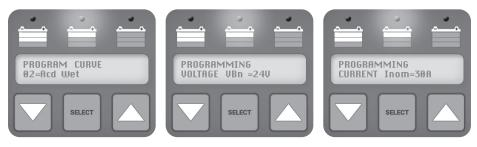
After selecting the parameter, you want to change, press **SELECT** to activate the option to edit the value (indicated by the red DL3 LED that turns on) and use the ▲ and ▼ keys to set the desired value.
