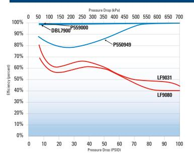
Tested per ISO 4548/12. Flow Rate - 150 lpm at 100°F / 38°C. Termination at 100 psid / 689.5 kPa. Efficiency time weighted average at 15 microns.
