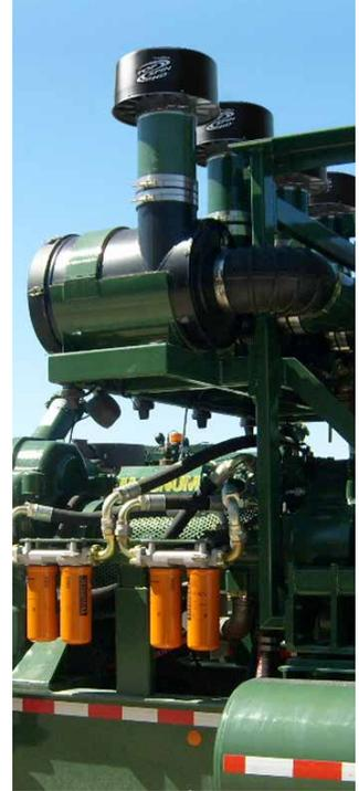
If dust, grit and dirt are a part of your daily operation, don't make your air cleaners do the job alone. Pre-cleaning the air entering the intake port can dramatically improve the life of air cleaners, and help avoid costly engine failure.
